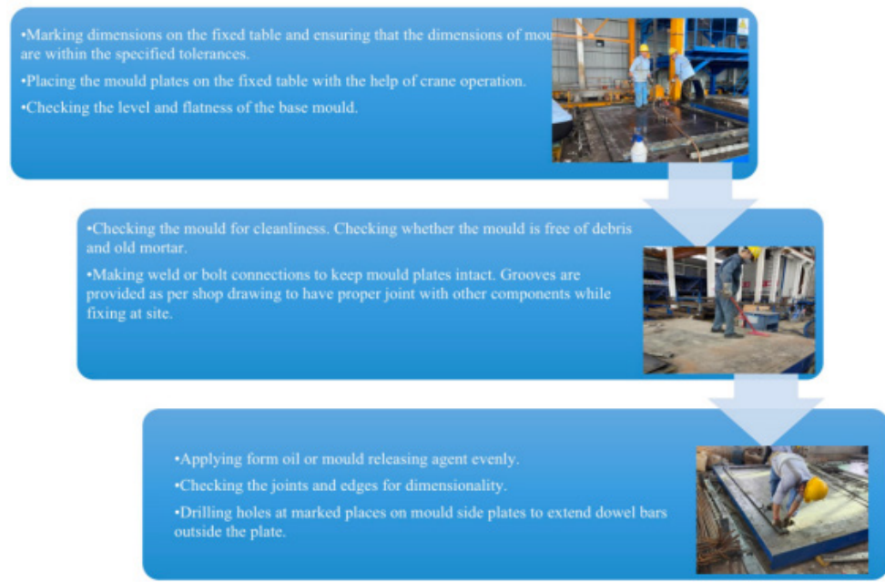
Fig. 1: Mould assembly and preparation of a prefabricated RC slab.
