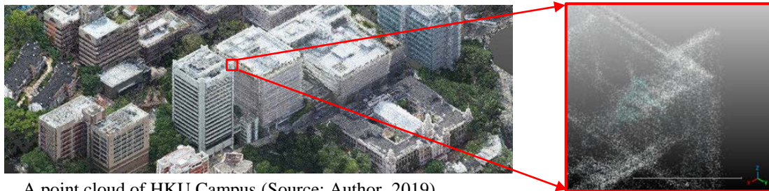
A point cloud of HKU Campus (Source: Author, 2019)
