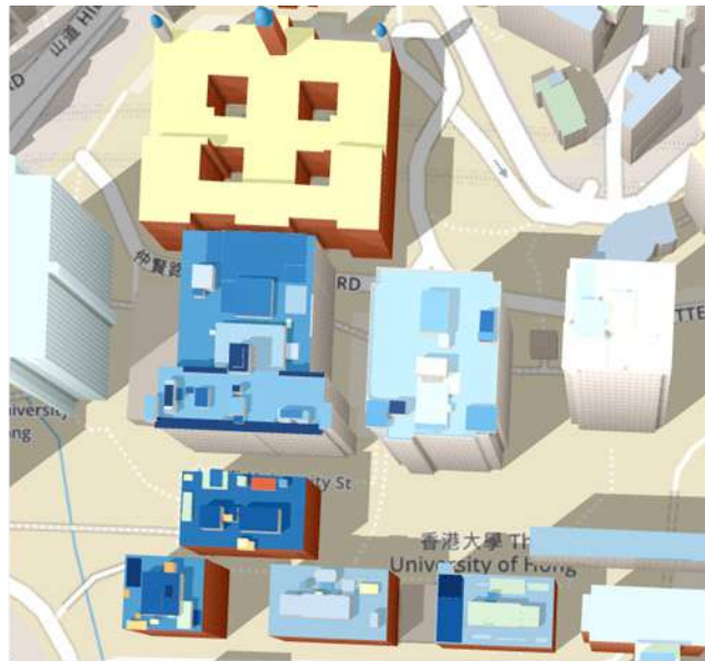
(b) 158 reconstructed rooftop elements using [2], where color indicates average reflectance (warmer = less)
