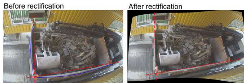
305 Fig. 4. Comparison between photos before and after distortion rectification.
