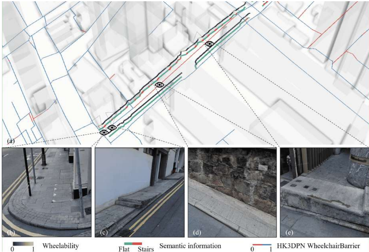
Figure 11: 3D view of segmented pedestrian results with wheelability index and semantic information. Subfigure d-e showcase zoomed-in photos captured by a digital camera of segments exhibiting varying wheelability levels.
