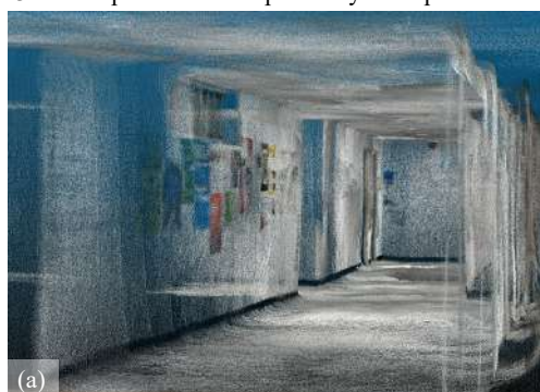
As-built data 3D color point clouds captured by smartphones
