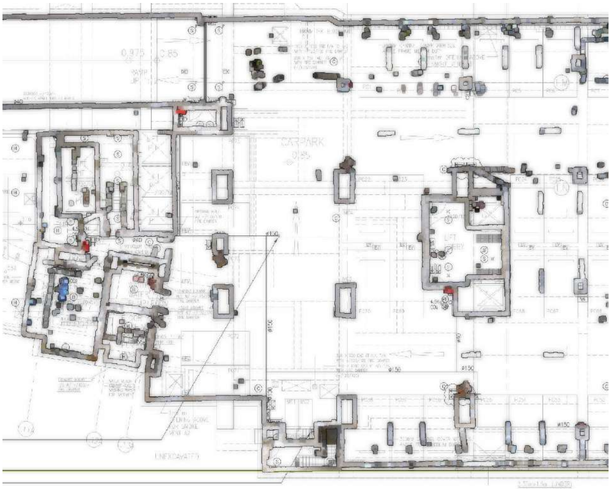
Figure 8. Registration result of 2D drawings with LiDAR point clouds. For better visualization, a sector along the z-axis is selected.
