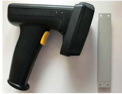
(b) Adopted UHF RFID reader and tag
