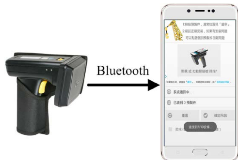
(i) RFID-to-BIM gateway
