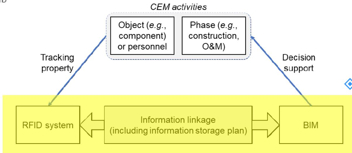
A conceptual model of linking RFID to BIM
