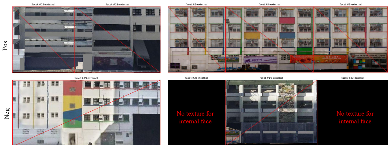
Figure 3. Paired textures for two decomposed parts in Case 1. Note: 'Pos' and 'Neg' denote the positive and negative symmetric sides of each part, respectively. The textures on the left correspond to the blue part shown in Figure 2, while those on the right correspond to the red part. Note that some facets on the symmetric planes are located internally within the building, and therefore no textures are projected onto them.
