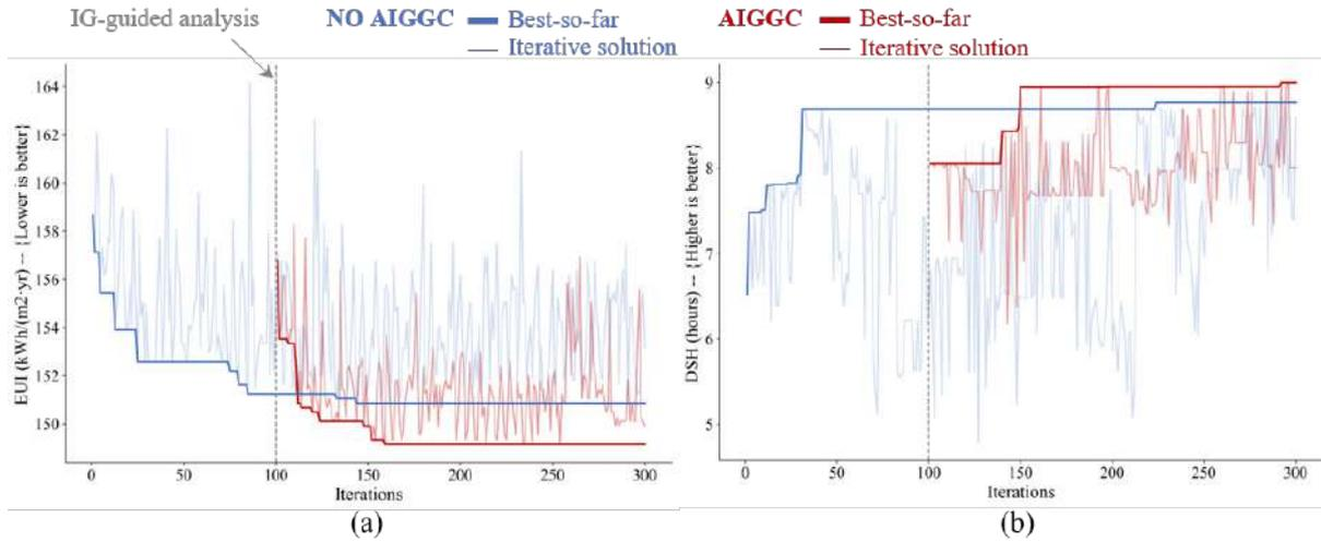
510 Figure 6. Convergence trend of optimization with and without AIGGC. (a) Case 1: Minimize  $EUI$ ; (b) Case 2: Maximize  $DSH$ .
