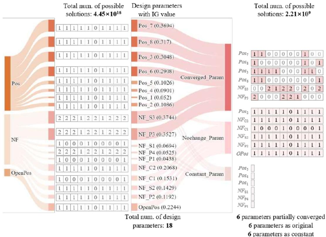
Figure 8. Detailed visualization of the design parameter convergence process for RBFOpt’s best performance solution in Case 2.
